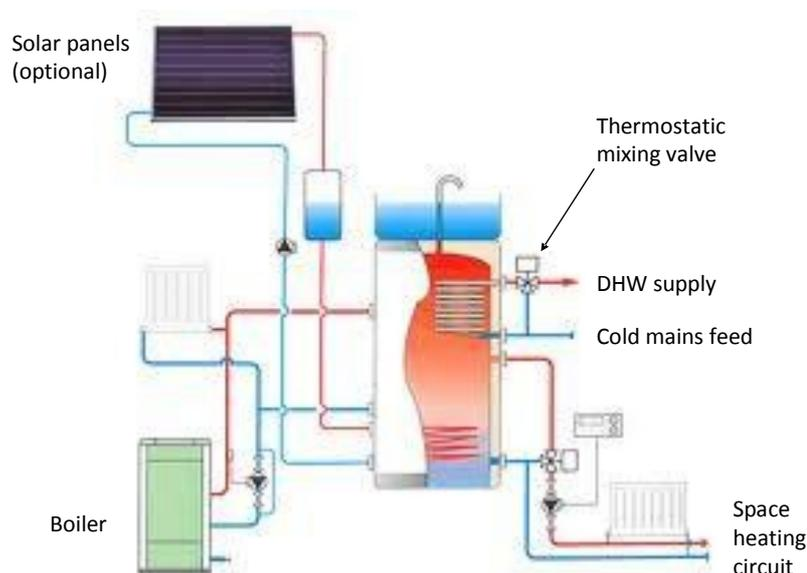
Figure 5-3: Integration of thermal store with existing heating and hot water system
