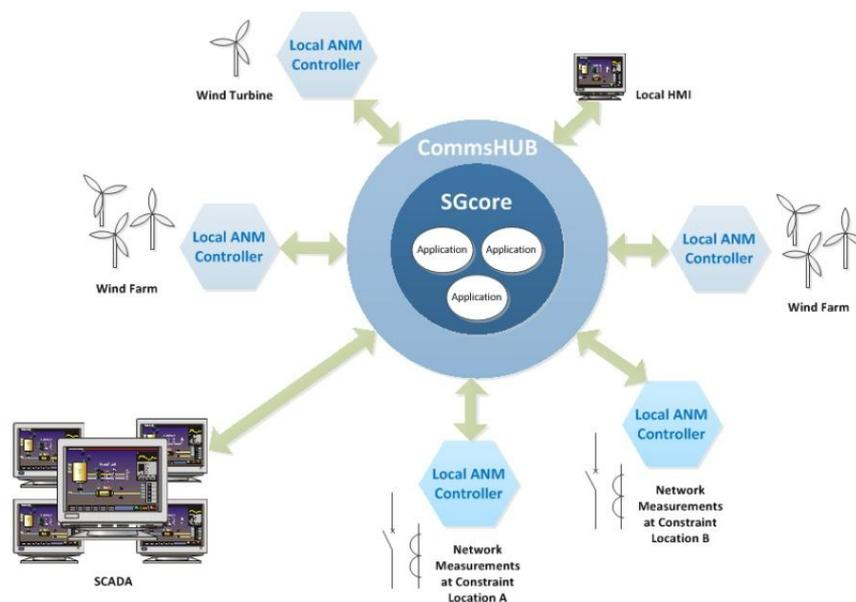
Figure 3-3: ANM system components
