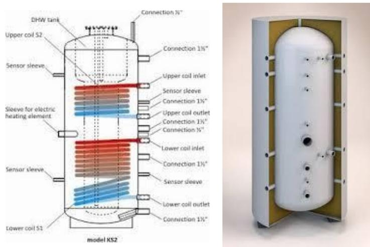
**Figure 5-2: Thermal store with heat exchange coils**
